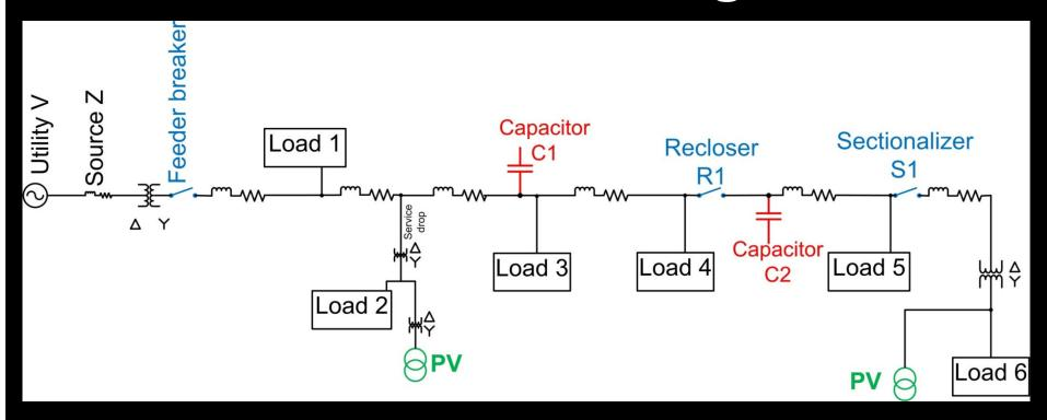
This is a generic distribution feeder. If part of the feeder is isolated by any of the blue switches from the "Utility V" at the left ("loss of mains"), any distributed generators, such as the PV plants shown in green, need to stop energizing the isolated part of the grid. If they don't, that section of the grid that's still energized is an *unintentional island*.
